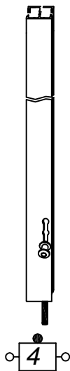
INTERMEDIATE POST: Pull Knob with Bottom Lock Rod with No Cylinders (Close Pattern Grilles)
