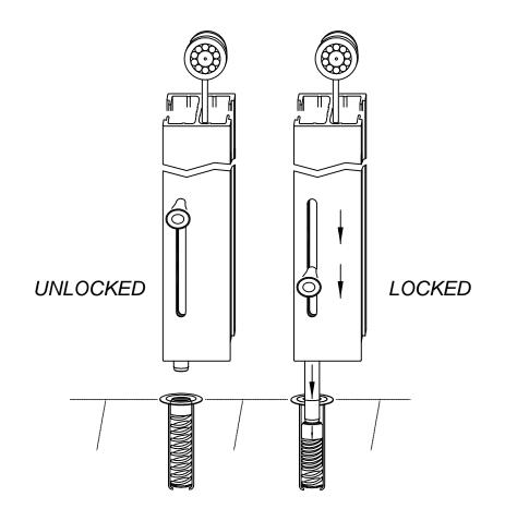
SLIDING CLOSURE FLOOR SOCKET INSTALLATION
