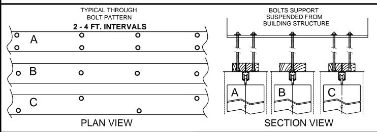
NOTE: HEADER WOOD OR STEEL SHALL BE DESIGNED TO SUPPORT THE STACKED LOAD OF THE GRILLE ANYWHERE ALONG THE TRACK INCLUDING THE POCKETS. ALL SUPPORTS ARE NOT ENGINEERED OR DESIGN BY DYNAFLAIR THE ABOVE DETAILS ARE SUGESTED METHODS OF ATTACHMENT AND ARE REFERENCE ONLY.
