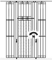
ROTATE THUMBTURN (OR LEVER) THROUGH 90 DEGREES OF TRAVEL TO RELEASE HOOKBOLT
