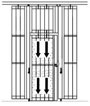
MAN DOOR INSERT DROPS DOWN FREE OF FOLDING PANEL SECTIONS ABOVE
