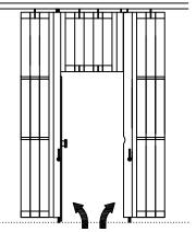
MAN DOOR INSERT SWINGS OUT ON A VERTICAL AXIS IN THE DIRECTION OF EGRESS
